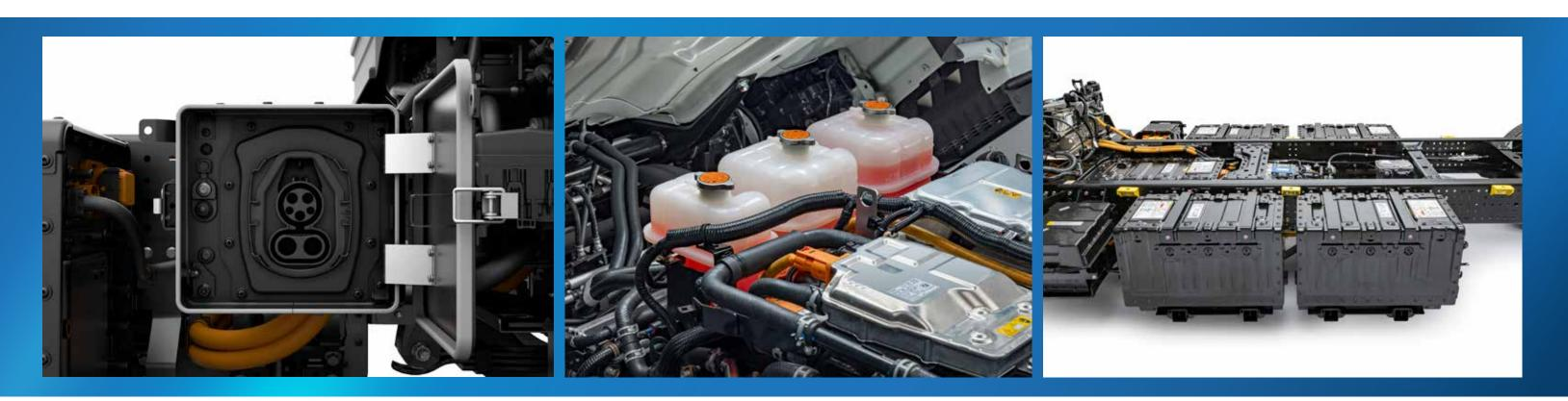
The NRR EV's high voltage batteries and electric drive motor are cooled by a water-based coolant. Without sufficient cooling, drive motor output will decrease; high voltage battery output will drop; charging time will increase.
